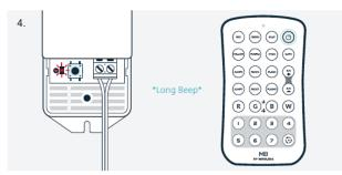
Press the black Sync Button on the receiver once and the the Power Indicator LED will remain static, then quickly press any button on the remote and the Power Indicator LED will flash faster then continue flashing at a slower pace as before. The remote is synced. (To reset the receiver and try again, press and hold the sync button until it beeps twice (about 10 seconds). The receiver is reset)
