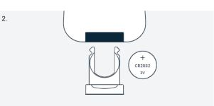
Open the tray on the back of the remote and make sure the battery doesn't have the protective plastic.
